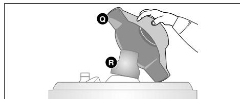
extract the flue deflector and clean the flue with a metal brush, taking care not to damage its coating with blows.
