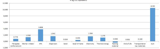
The chart shows that the XPS contributes the greatest proportion of global warming potential per declared unit, which is above all attributable to the specific production process (see Chapter 2.5). In comparison, the processes relevant for production (Module A3) make only a small contribution to GWP as the preproducts are together already responsible for 87 % of greenhouse gas emissions.
