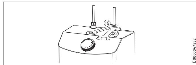
Match up the colour coding on the tap water connections and the appliance:
