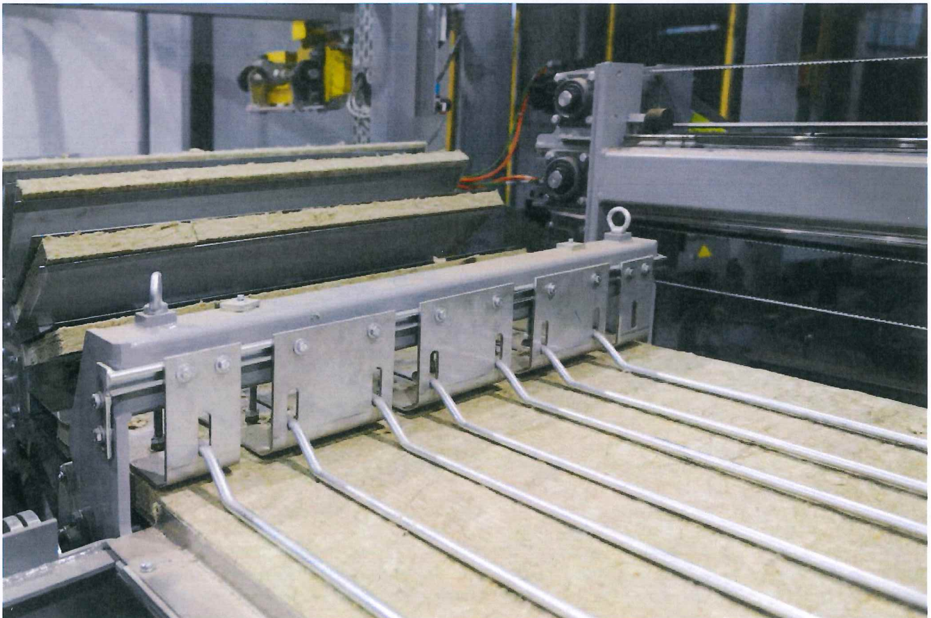
Photo 2 - Thermal insulating pads prepared at carousel
