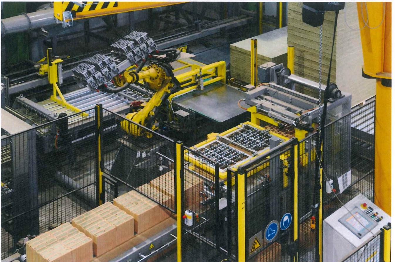
Photo 4 - Inserting thermal insulation into brick blocks
