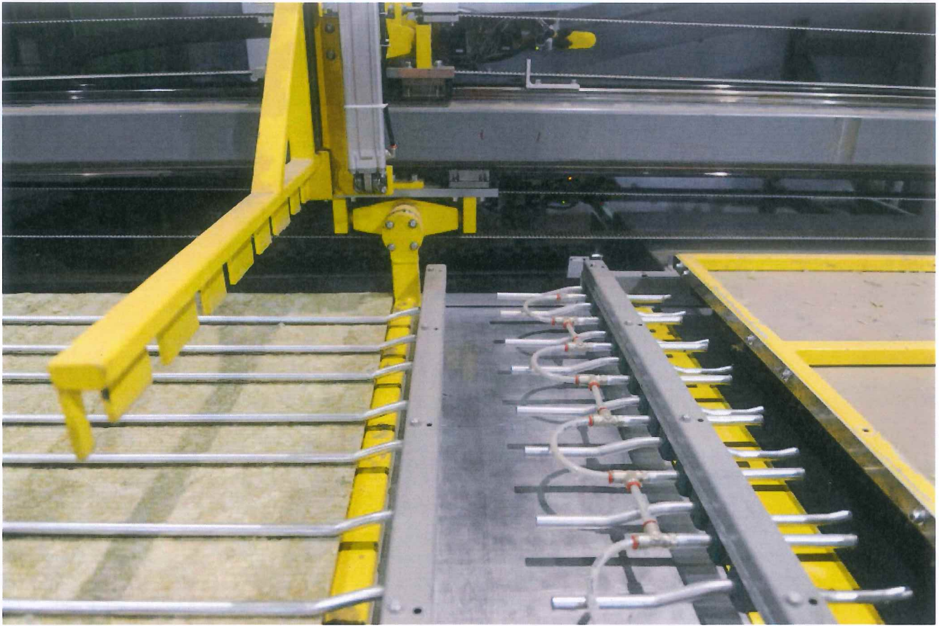
Photo 1 - Water jet cutting of mineral wool thermal insulation boards for pads inserted into bricks
