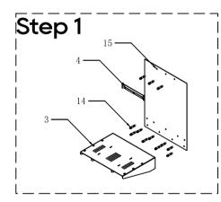
Fix the Wall Mounting Base and Wall Mounting Plate to wall with expansion screws by Positioning Board.
