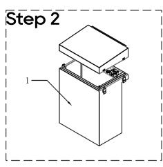
Untwist latches to remove the top cover of main cabinet
