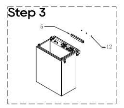
Fix the Wall Mounting Adapter to Cabinet with M4 Screws
