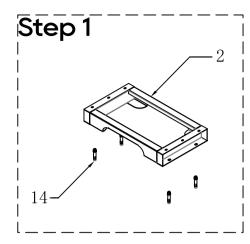
Fix the Floor Mounting Base with expansion screws
