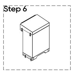
Place and lock the top cover to main cabinet by twisting the latches.
