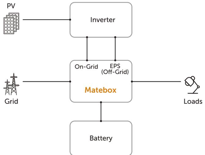
For the new X-ESS G4, we get rid of the complicated wiring work by laying all the wires in the Matebox. All you need to do is just to install one module on the top of another, and connect all the cables which are already well-sorted in the Matebox in different ports.
