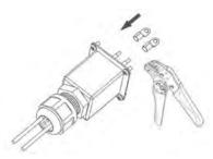
**Step 2:** Install the battery power connector
