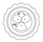
Assemble the AC connector and make sure that the rib of the terminal block and the groove on the housing engage perfectly until a 'click' is heard or felt.
