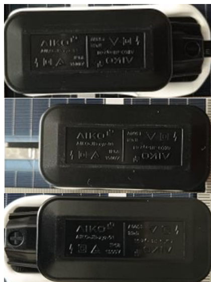
Fig. 5: detail view of closed junction box
