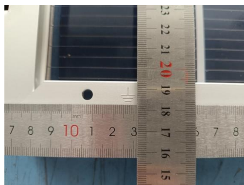
Fig. 9: detail view of grounding hole
