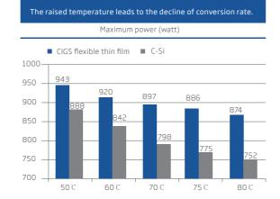
rature of module is basically larger than the standard test temperature 25 C (a  $g\,60$  C in summer). The flexible thin film module is low in temperature coefficient
