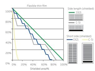
The electricity generation performance remains remarkable when the bypass diode set between two battery slices of every flexible thin film module is shielded.
